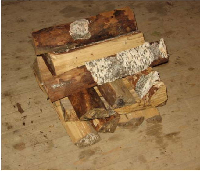
Fig. 17. Birch chocks, 13 pieces. The weight of 12,8 kg, moisture is unknown.
